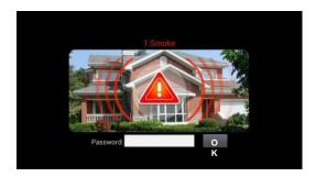
☐You can see the sensor No. and type in Red, shown at the top of the screen. For example, "2: Smoke" indicates that a smoke sensor in zone 2 is triggered. To stop alarm, input the password (the default password is 1234).
